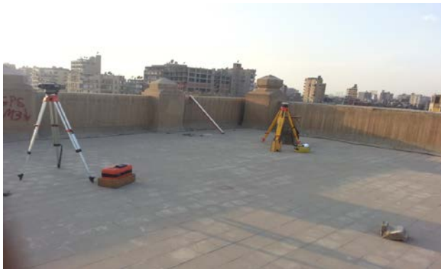
Fig. 3. The optical precise level settled in front of the GPS receiver about 5 meters away in order to have the staff readings above the antenna exactly
